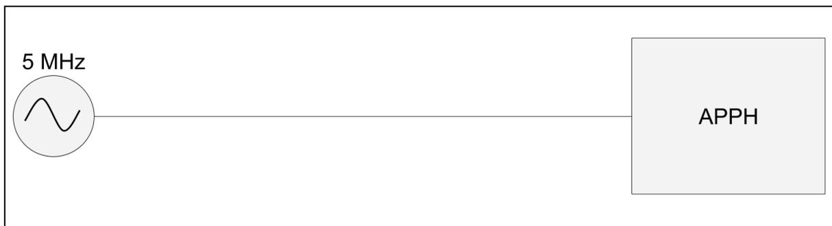
*Figure 1. Measuring the synthesizer output directly.*
