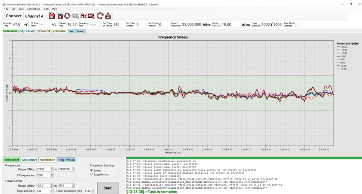
2. Run an Adjustment with default parameters across the full device frequency range and a displayed tolerance of +/- 1dB. [for details see 'Adjustment/Verification' section within the User Guide]
