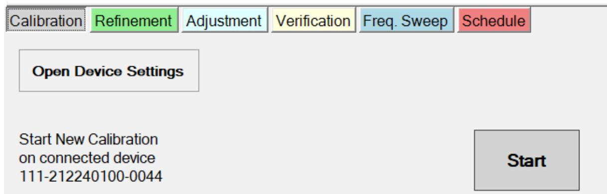
3. Switch to the refinement tab and ensure the tolerance is set to 0.35dB, Additional Points is set to '3' and the frequency range to calibrate matches the calibrated frequency range of the DUT model (the frequency range can be verified by clicking 'Open Device Settings' on the 'Calibration' tab).
