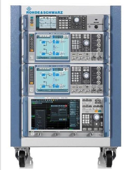
The system consist of Analog SG SMA100A as shared LO, 2 units VSG SMW200A + VNA for time and phase calibration. Plus cables adapters and test bench.
