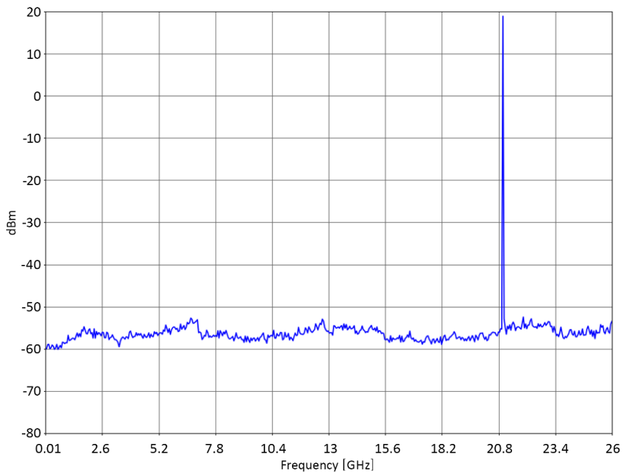
Figure 5: Wideband Spectrum at 21 GHz output
