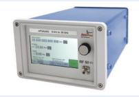
he AnaPico APSINxx-series signal generators with 12 or 20 GHz upper frequency range are now available with FILT and PE2 options. The FILT option provides a harmonic level of -60 dBm in the X- and Ku-Band frequency ranges while keeping the maximum power level at +25 dBm. The PE2 option includes a mechanical step attenuator that allows the signal generator to operate down to an input power of -120 dBm.
