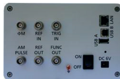
Figure 2 External modulation signals are provided through the rear panel connectors.
