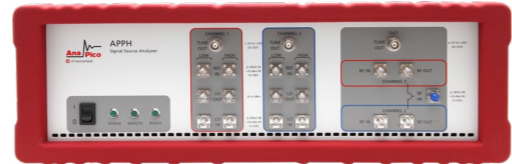
Option LO offers access to internal LO's and individual RF channels
