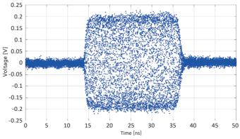
APMS40G-ULN 25 ns Pulse Modulation – 40 GHz Carrier Frequency
