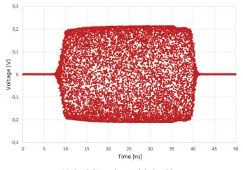
APLC: 10 GHz pulse modulation 30 ns
