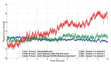
Channel-to-Channel Phase Stability under Different Test Conditions
