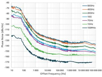
APHSP: Phase noise at different frequencies. Power level +10 dBm, with option LN(+)
