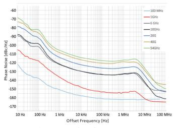
APLC: Phase noise at different frequencies, power +10 dBm, with option LN
